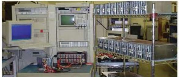
*Quick Connect Fixture on production floor*
