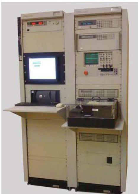
Tester with Test Fixture and UUT
