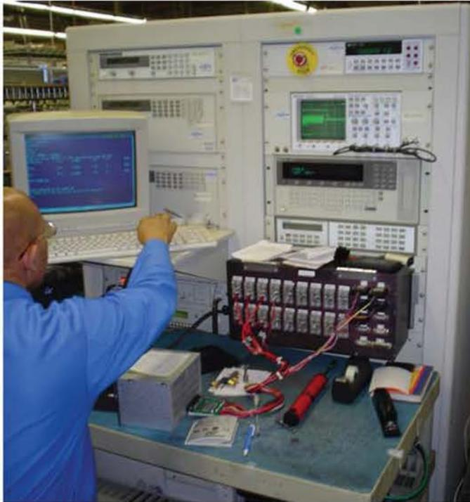
*Quick Connect Fixture with UUT*
