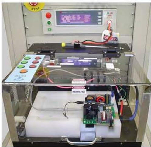
*Close-Up Test Fixture with UUT*
