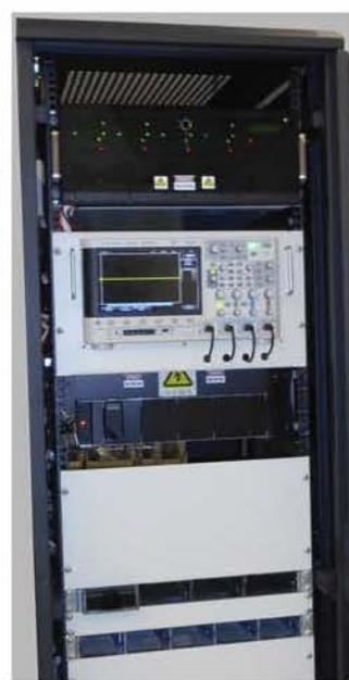
*Fixture with added HV Loads and Scope*
