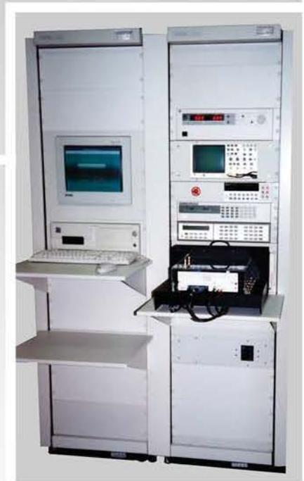
*Test Fixture on ATE*
