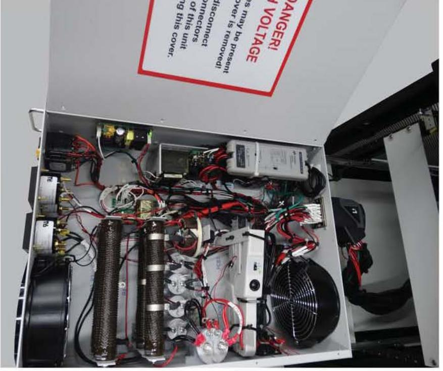
*Interface Unit with Top Removed showing Differential and Current Probes, Resistive Loads, Relays etc.*
