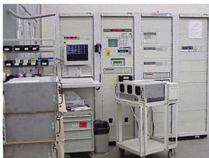
*Cart and Cable Test Fixture with UUT*
