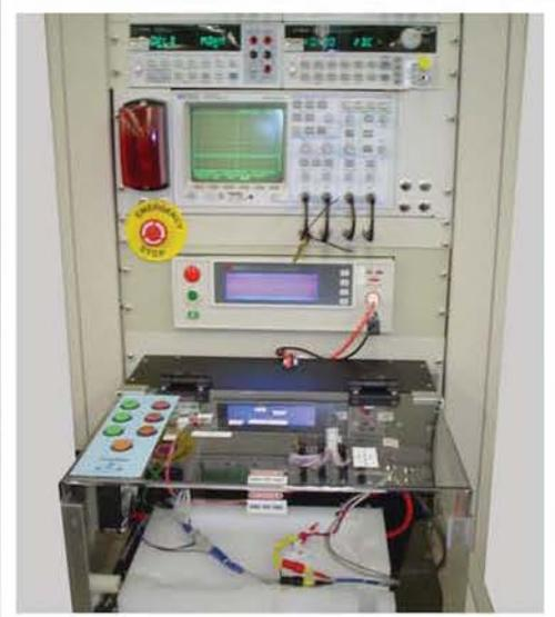
*Test Fixture connected to HIPOT*
