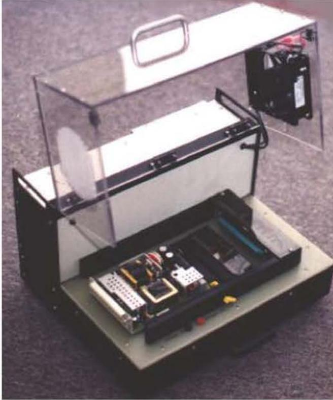
*FineTest Test Fixture Kit with UUT*
