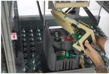
*Adapter Palte to connect to UUT*
