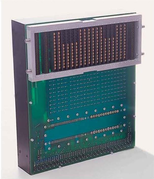
Rear view of DCA Test Fixture
