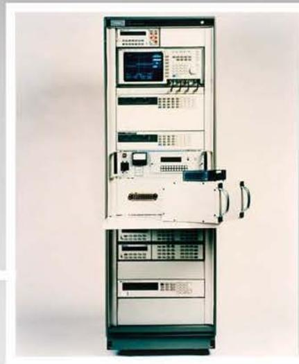
*Plug-In UUT Test Fixture*
