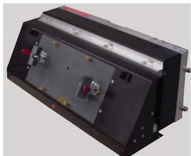
*Side view Pogo-Pin Board Test Fixture*
