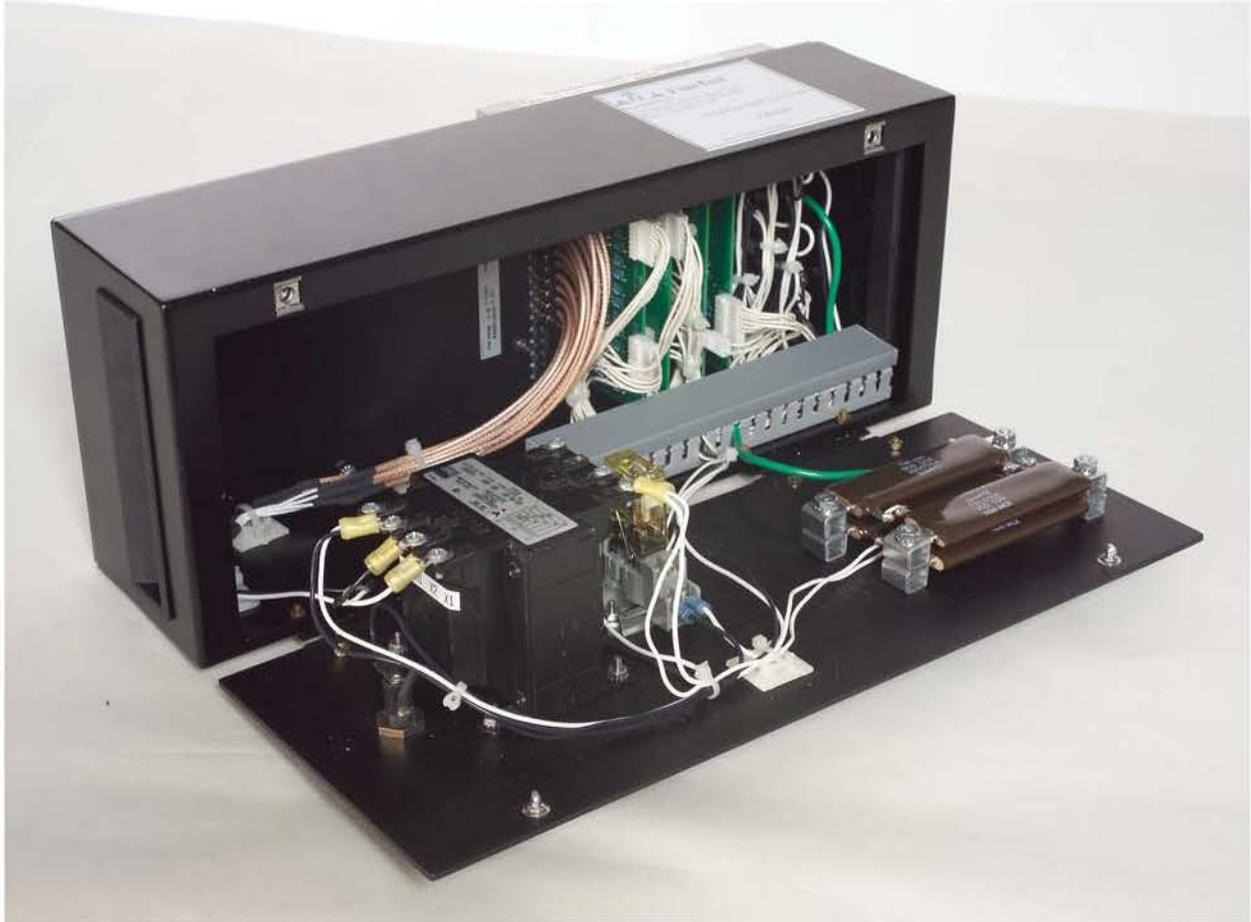
*Self-Test Fixture with rear cover open*
