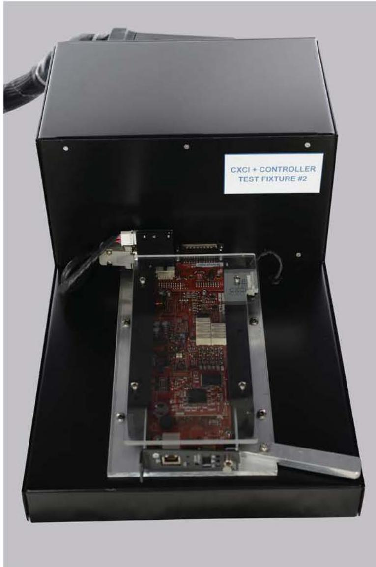
Close-Up Test Fixture with a UUT
