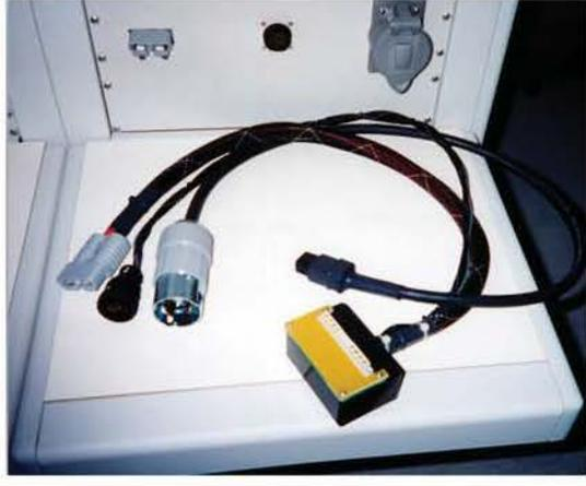
*Cable to UUT Test Fixture*
