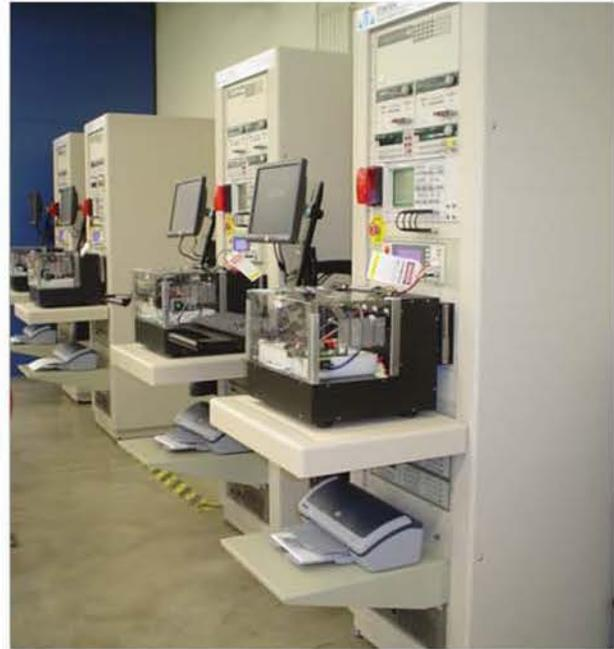
*Duplicate Test Fixtures on production floor*
