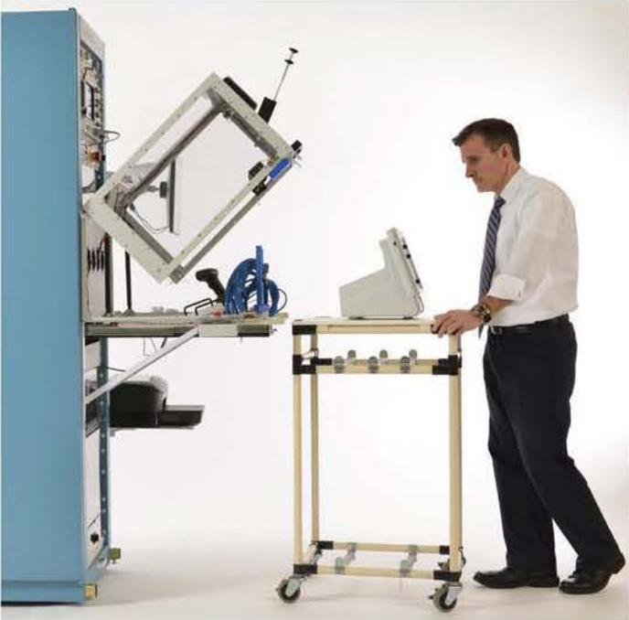
Rolling-In a UUT with a Cart
