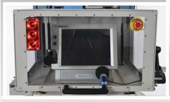
Safety Cover with Flashing Lamp
