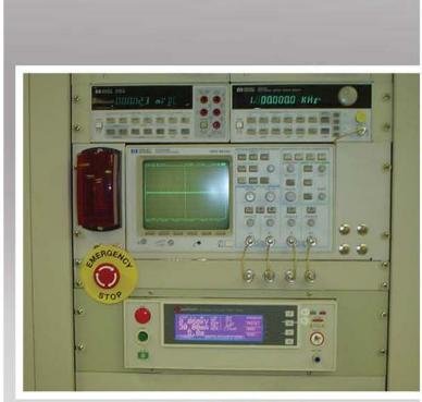
Close-Up of HIPOT unit and Flashing Safety Lamp
