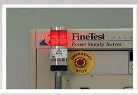
Close-Up of Flashing Safety Lamp
