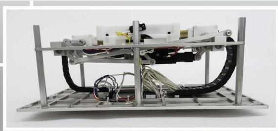
Internal Side View showing Linear Actuator to make connection to UUT
