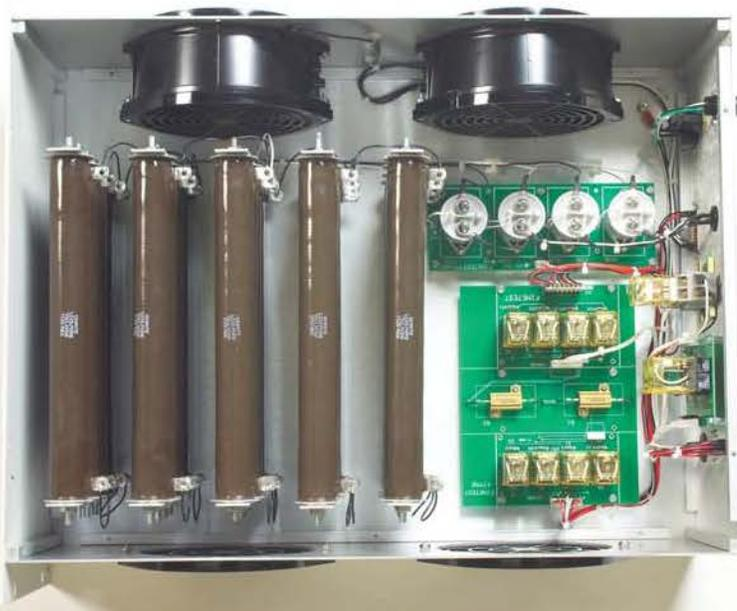
*Top View showing Resistors and High Power Relays*
