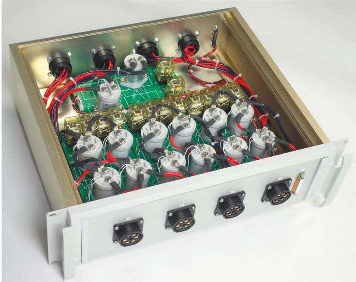
*Top View with Cover Removed showing High Voltage/ High Current Power Relays*
