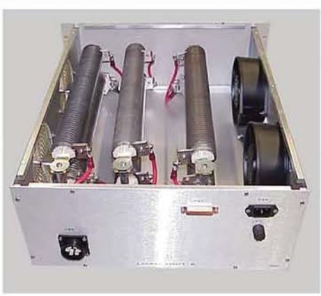
*Rear view of Resistive Load Unit*
