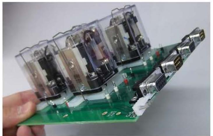
Close-Up of one Relay Board showing DB9 Connectors and Test Points
