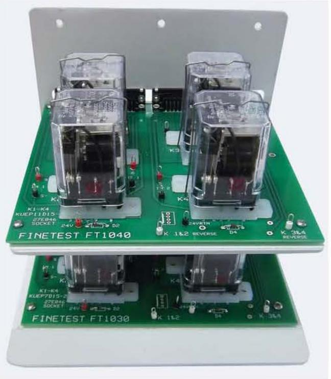
Cover Removed showing Relay Boards
